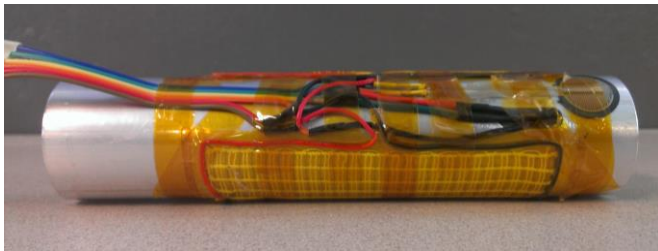
Figure 5 – Tube body with electric components taped in place before silicone coating
