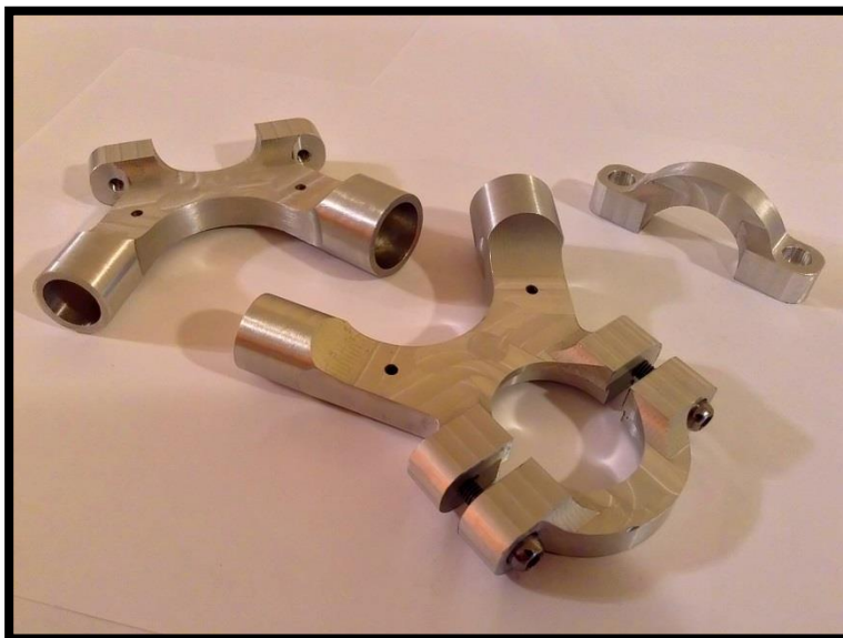
FIGURE 15: REAR DROPOUTS BEFORE BEING WELDED TO THE FRAME.
